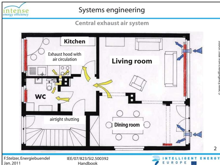
The ventilation system is a central part of a passive house. Normally only systems with heat recovery are used. This is the system with the most influence on comfort, hygiene, heating and cooling. Also building physics is influenced.
