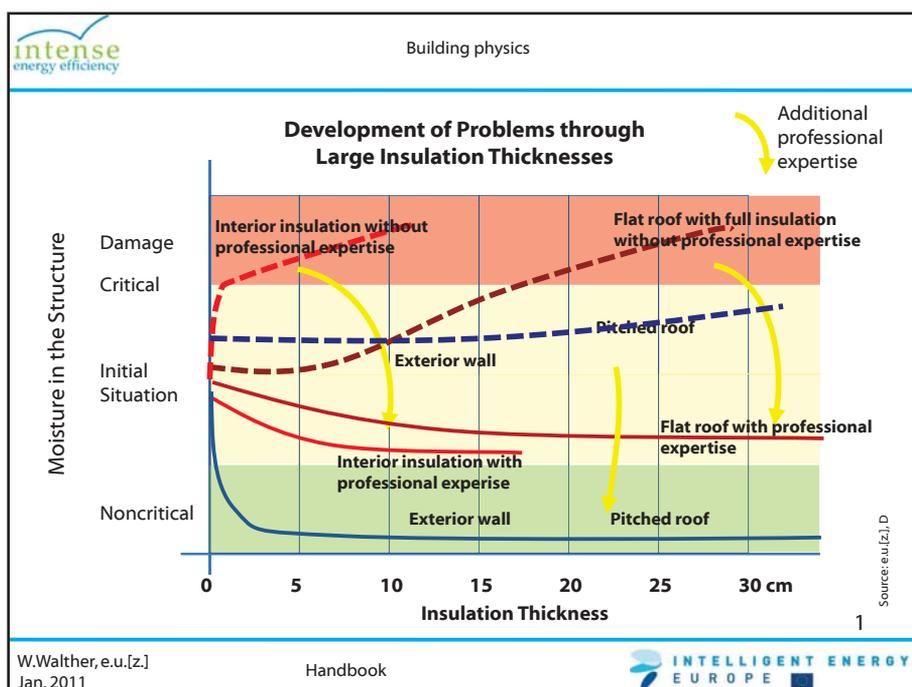
Despite large insulation thicknesses, the building envelope of the passive house can be implemented without any risks. However, this requires professional expertise with regard to mould prevention, thermal bridges, diffusion, and airtightness of the building envelope. The large insulation thicknesses of the building envelope differ in their impact on the moisture behaviour within the various structural components.
