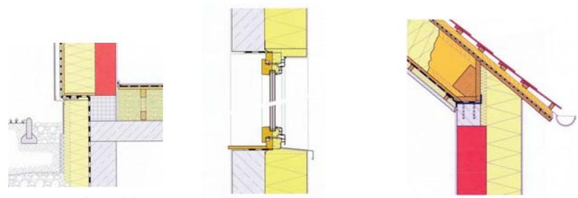
Separating the cold basement ceiling through a "levelling block" with very low thermal conductivity
