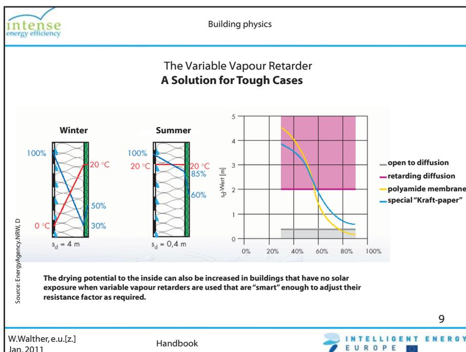
Many building materials have an  $s_d$ -value independent of relative humidity. They are shown as a horizontal line (color column) in the figure. Wood and wood products, vapour retarder membranes based on paper as well as polyamide membranes and polypropylene liners change their  $s_d$ -value depending on the relative humidity.
