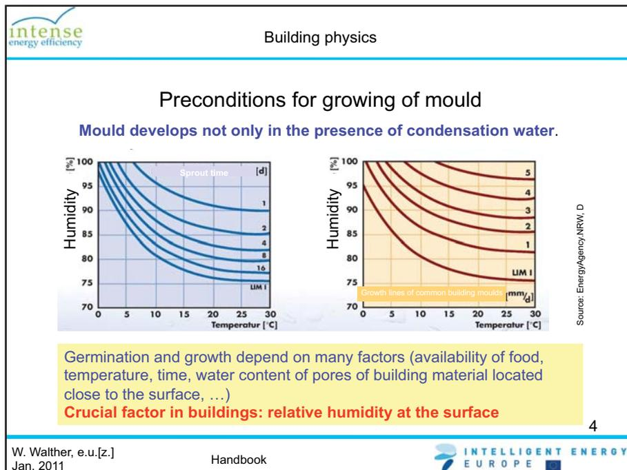
Mould germination and growth rate depend on the temperature, but especially on the relative humidity of the surface of a given material. To be safe from mold growth, relative humidity levels need to be at least below about 75%. At temperatures of about 10 °C, the growth conditions are achieved at 80% r.h. (see graph).
