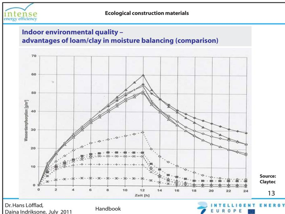
This slide shows the advantages of loam and clay in moisture balancing in relation to indoor environmental quality. The chart shows the water vapour absorption [ $\text{g}/\text{m}^2$ ] of different finishing materials. All samples were tested in the same climate for 12 hours. The absorption was measured and the samples were dried under the same conditions. All finishing surfaces with clay and casein paint show fast and high moisture absorption.
