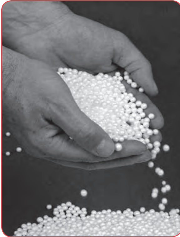
Fig. 3. Expanded polystyrene (EPS) is a synthetic insulation material | Image: © Nikecell
