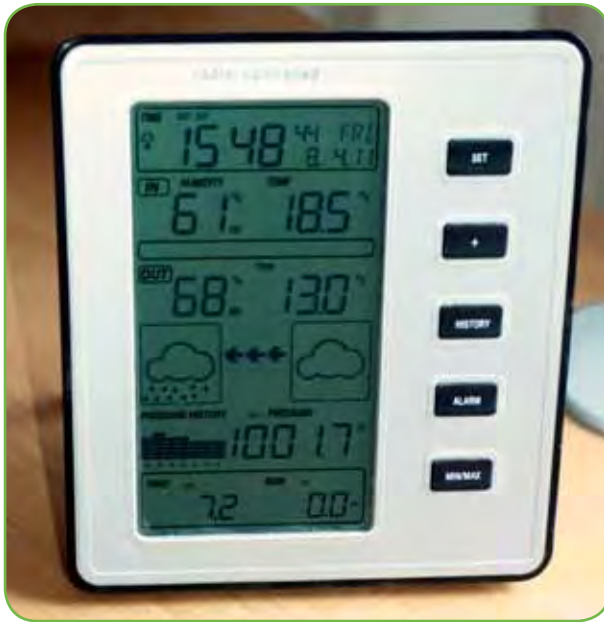
Fig. 2. Hygrometers help you to keep an eye on the indoor humidity. In this example it is more than 60%, time to open the windows for a couple of minutes. Image: © Philipp Engewald.
