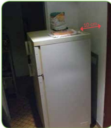
Fig. 5. A gap between furniture or larger appliances and the wall allows air circulation Image: © Philipp Engewald
